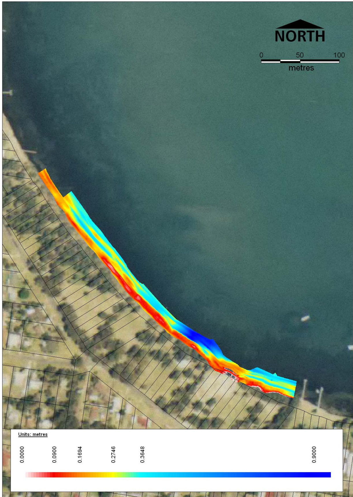
Figure 2.13 Depth of unconsolidated (organic) sediment in Bonnell's Bay (derived from survey by Cadman Consultant, 2004)
