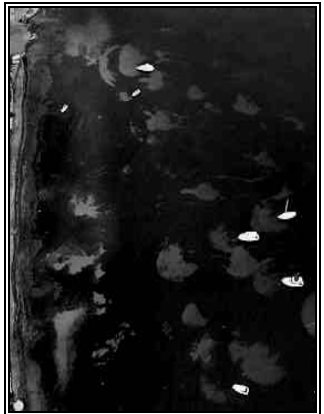
Figure 4.2 Oblique Aerial Photographs Illustrating the Damage to Seagrass Beds caused by Mooring Chains
